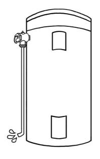
**Marning:** Never replace the relief valve with one of a higher pressure rating.
