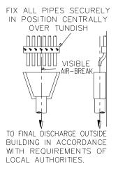
TPR Valve Drain Line Common Discharge Point
