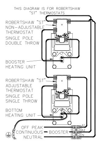
Top thermostat – fixed setting Bottom thermostat – tradesperson adjustable 60°C. min 60°C, max 70°C.
