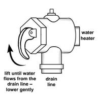
If water does not flow freely from the drain line when the lever is lifted, then the water heater must be checked. Phone Rheem Service or their nearest Accredited Service Agent to arrange for an inspection.
