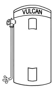
⚠ Warning: Never replace the relief valve with one of a higher pressure rating.
