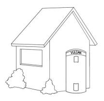
The water heater is to be installed at ground or floor level and must stand vertically upright on a stable base as acceptable to local authorities. The base of the water heater is made of corrosion resistant material, and it may be placed directly in contact with the supporting surface. It is not necessary to allow for free air circulation under the base of the water heater.
