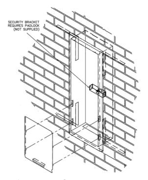
The installation position of the Rheem Continuous Flow unit must comply with AS 5601. This should be considered when choosing the position of the Recess Box.
