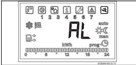
Fig. 71 Showing all the display's segments
