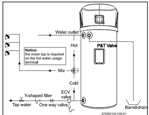
Fig. 9 Typical installation
