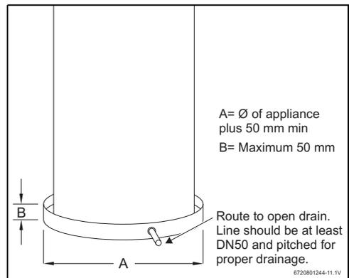
Fig. 8 Water heater support as specified in AS3500.4
