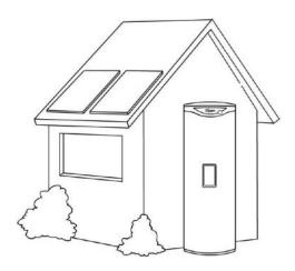
**Note:** The water heater should not be placed in direct contact with a concrete surface that is less than two months old and not fully cured as this may attack the metal coating of the water heater base. A moisture barrier should be used between the two surfaces in this instance.
