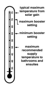
If this water heater is installed with an in-series storage booster, then this requirement of AS 3498 can be satisfied provided the storage booster is energised and its thermostat setting is 60°C or higher.
