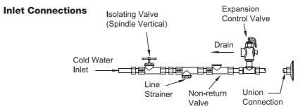
**Note:** a combined isolating valve/non-return valve/line strainer may be used. Expansion valve only required where local regulations demand although it is recommended in areas where the water saturation index is above 0.40.
