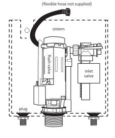
All measurements are in millimetres. Height dimensions are to base of pan. Make allowance for bedding. This toilet suite can be set up as either Bottom Entry Inlet or Back Entry Inlet.
