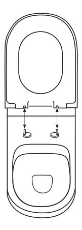
To fit seat, slide seat down onto stainless steel pins.
